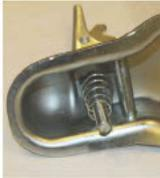
**Step Three -** Slide ball clamp up on spade bolt with cupped part facing upward and toward coupler ball pocket. Back lip of ball clamp is to be up and over the coupler re-inforcing bar.
