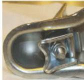
**Step Six -** Slide U shaped washer on the spade bolt. Make sure the washer remains in this orientation.
