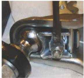
Once instructions above are completed, coupler is adjusted properly and coupler is in the closed/engaged position the bottom of coupler and proper size hitch ball in the coupler ball pocket should look like photo to right. It is important that the u shape washer remain in this orientation. Also after adjustment there should never be less than a full thread exposed on the spade bolt below the bottom of the nut.
