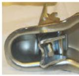
**Step Four -** Slide ball clamp washer on the spade bolt with the flat side of washer facing forward.
